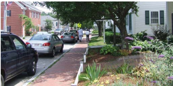
Sidewalk protected by curb and on-street parking on Route 6A in Barnstable.
