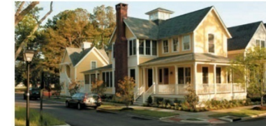
3.3 A successful corner lot creates a strong frontage along both the primary and secondary streets. Landscaping elements soften the hard edges of the building along the front and side setbacks.
